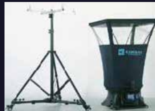
Portable stand: extends up to 6.9' from top to base
