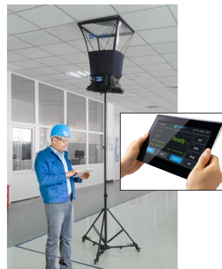
The Bluetooth® feature can send data to any Android-based device
