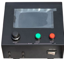
Built-in micromanometer with pre-programmed testing standards and motor speed controls
