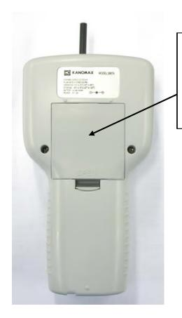
**Battery Compartment**Use four (4) AA rechargeable batteries or alkaline batteries. Operating hours by battery power are only ensured when using the supplied Ni-MH batteries.
