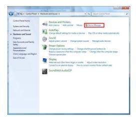
5)After opening the Device Manager window, confirm that "KANOMAX DIGITAL DUST MONITOR MODEL 3443" is listed in "Other Device" and right-click it.
