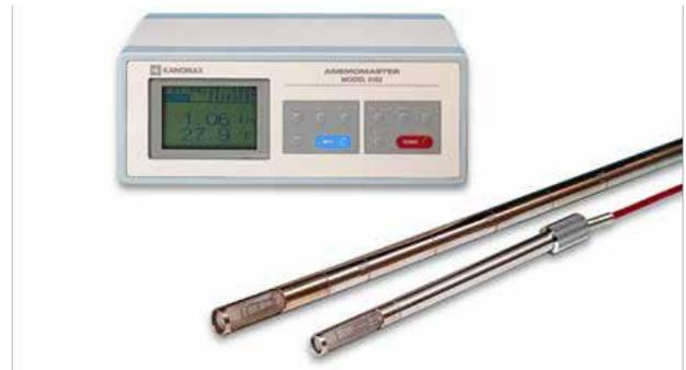
Model 6162 High Temperature Anemometer
