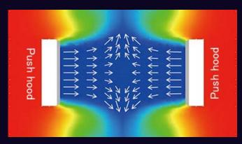
The purified, uniformed laminar airflow having the same vector collide at the center between the two push hoods and are pushed out horizontally. As a result, the intervening zone between the push hoods is kept clean.
