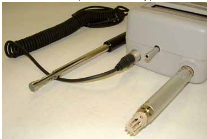
GEO- \alpha with the T/H probe and Air velocity probe installed
